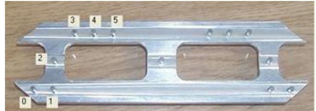
Figure 5.6–MOI Jig Mounting Pin Locations
