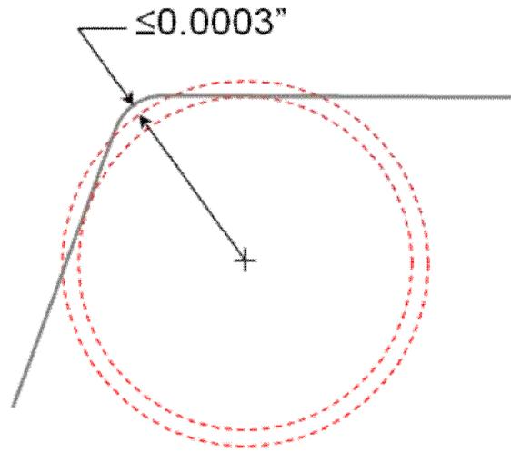
**Figure B.5:** Maximum protrusion
