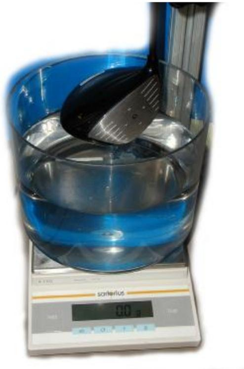
**Figure 5.4 – Tared Electronic Scale with Water-Filled Container Ready of Clubhead Immersion**
